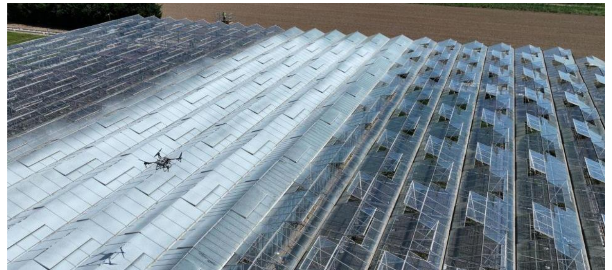
A sprayer drone from Norfolk firm Crop Angel whitewashing greenhouses in Lincolnshire (Image: Crop Angel, www.cropangel.com )
